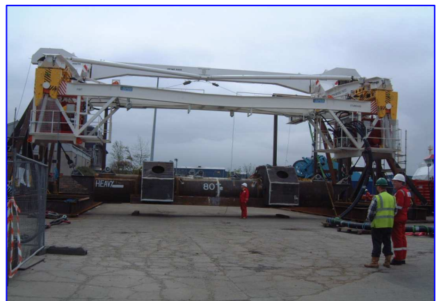
Onshore Testing of Large Offshore Gantry Crane
